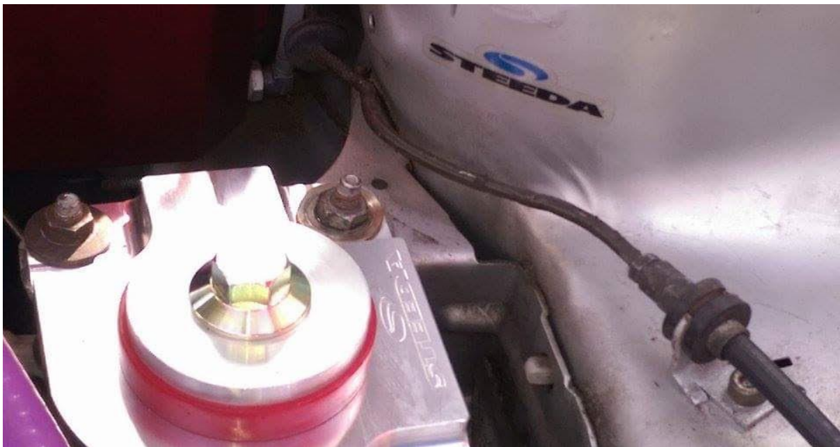
The gearbox mount provided by Steeda UK . Photograph reproduced with permission from Alison Kozary.
